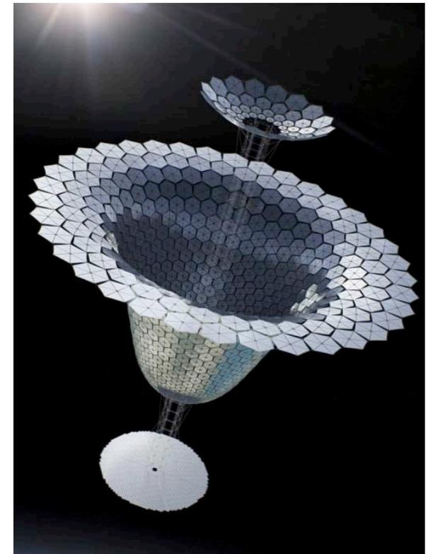
Each Alpha Mark IIIA is 9,800 tonnes (to GEO) - For output of 2 Gwatt continuous power
