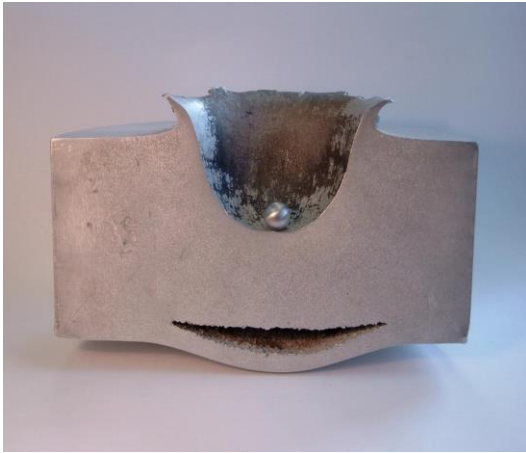
Figure 5: Impact crater from experiment of sending aluminium sphere into a block of aluminium. [10]
